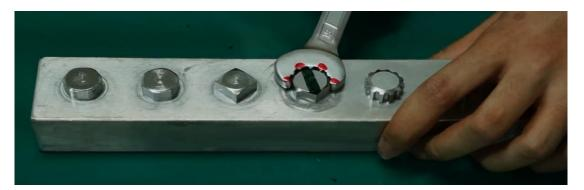
In this way, the stress equally spreads on four-point, each point takes less pressure than before which can reduce the chance of deforming. Also because of its four point fit-in and smaller open end side designs, those shorten the pull back distance which can drive nuts faster.
