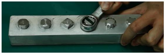
The unclosed-ring design upgrades the open-end side's jaw from its original two-point fit- in to four-point fit-in.
